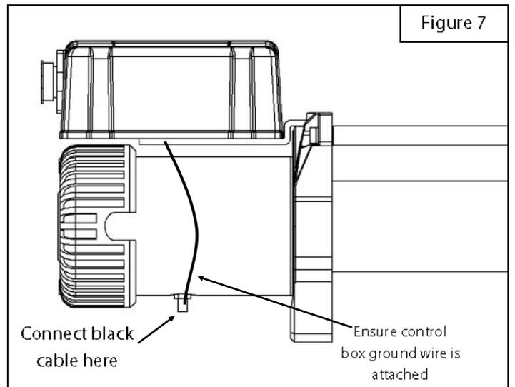
10. Connect your remote and rotate the drum on the winch outward until the end of the cable is facing the front. **Ensure that the rope is routed under the winch (underwound).** Damage will occur if not underwound. Carefully pull the cable through the fairlead. Connect your hook to the fairlead with the clevis pin and cotter pin. See **Figure 8 & 9**.
